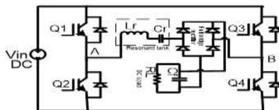
Figure 1. The typical configuration of the (SRC)
