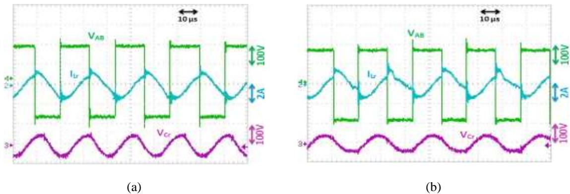
Figure 9. Measured waveforms of the resonant tank input voltage  $V_{AB}$ , resonant inductor current  $i_{Lr}$  and resonant capacitor voltage  $V_{cr}$  of conventional SRC at  $V_{in}=180$  and (a)  $f_s=50$  kHz, (b)  $f_s=45$  kHz
