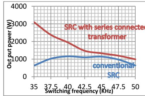
Figure 14. Measured converted output power at different switching frequencies
