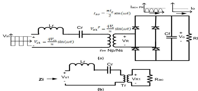
Figure 6. a) The stages and the variables of the converter topology. b) AC equivalent circuit with series connected transformer
