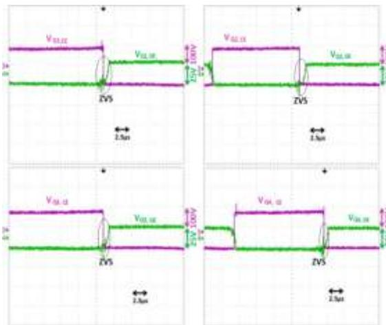
Figure 12. Measured waveforms of the gate voltage and collector voltage of all switches of the SRC with series connected transformer at  $V_{in}=180$  V and  $f_s=37.5$ kHz
