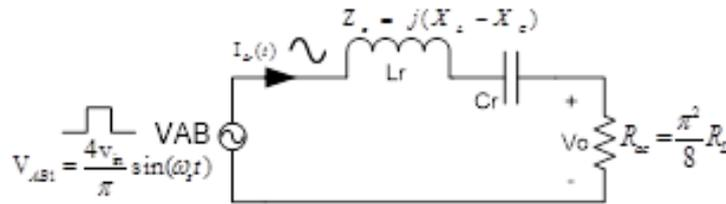
Figure 2. Equivalent circuit of the dc-dc series resonant converter
