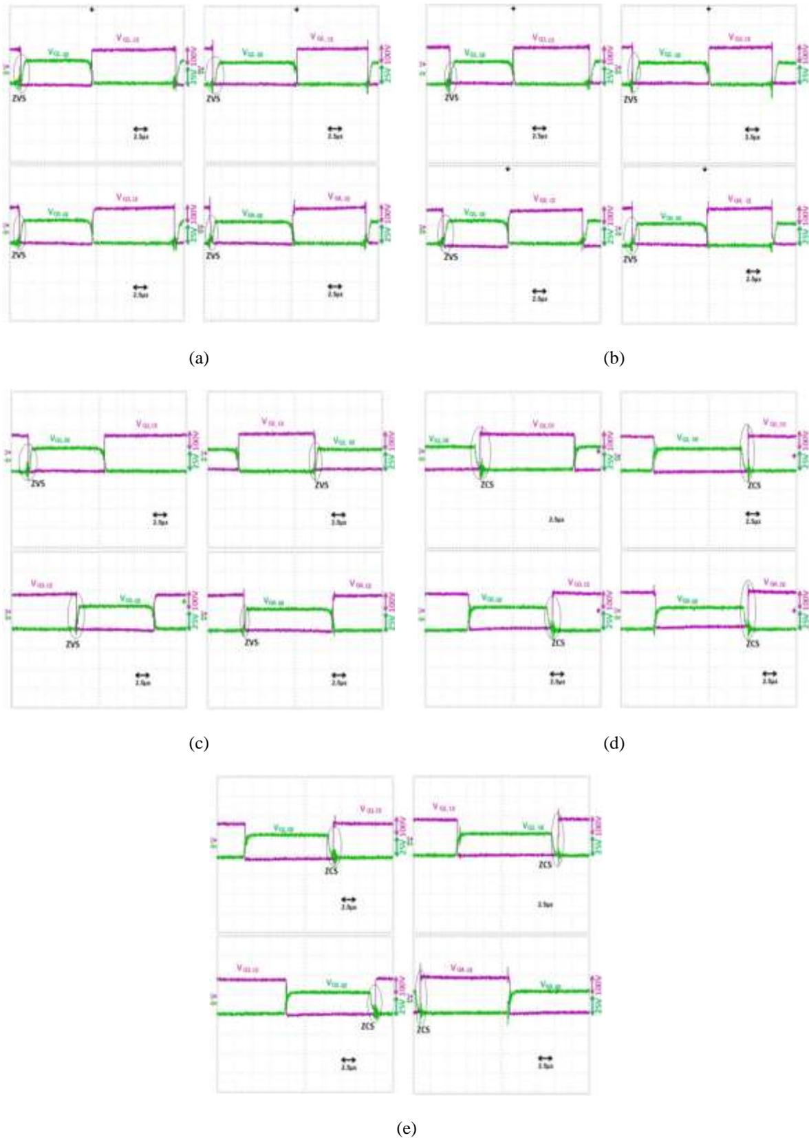
Figure 10. Measured waveforms of the gate voltage and collector voltage of all switches at  $V_{in}=180$  V and (a)  $f_s=50$  kHz, (b)  $f_s=45$  kHz, (c)  $f_s=42.5$  kHz, (d)  $f_s=40$  kHz, and (e)  $f_s=37.5$  kHz.
