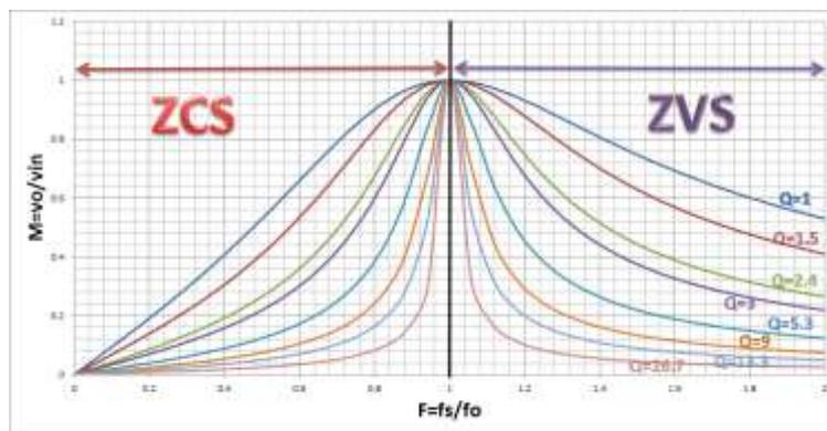
Figure 3. The gain characteristics of the SRC, for the range  $0 \leq F \leq 2$
