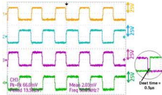
Figure 8. Gate driver signals at 50 kHz switching frequency
