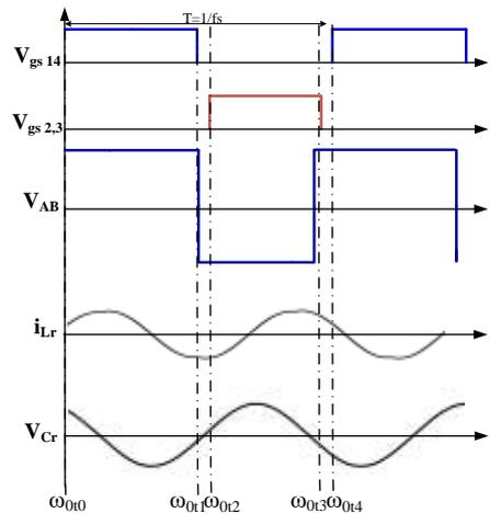
Figure 4. Operational waveforms of full-bridge (SRC) working above resonant
