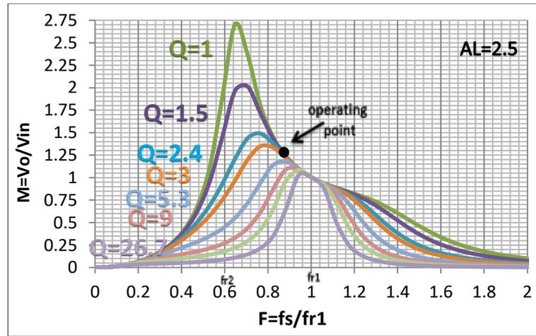
Figure 7. The gain characteristics of the SRC with the series step up HF, for the range  $0 \leq F \leq 2$ , and different load factor
